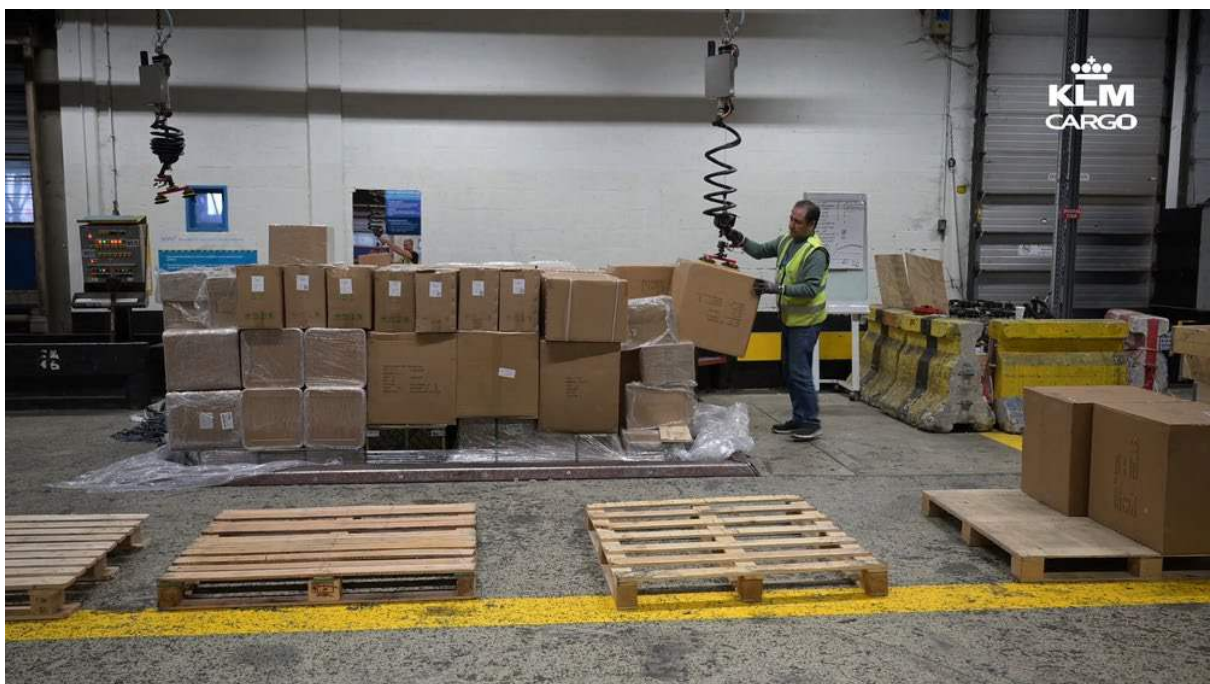
Vacuum lift operated at KLM Cargo Build-up & Break-down
